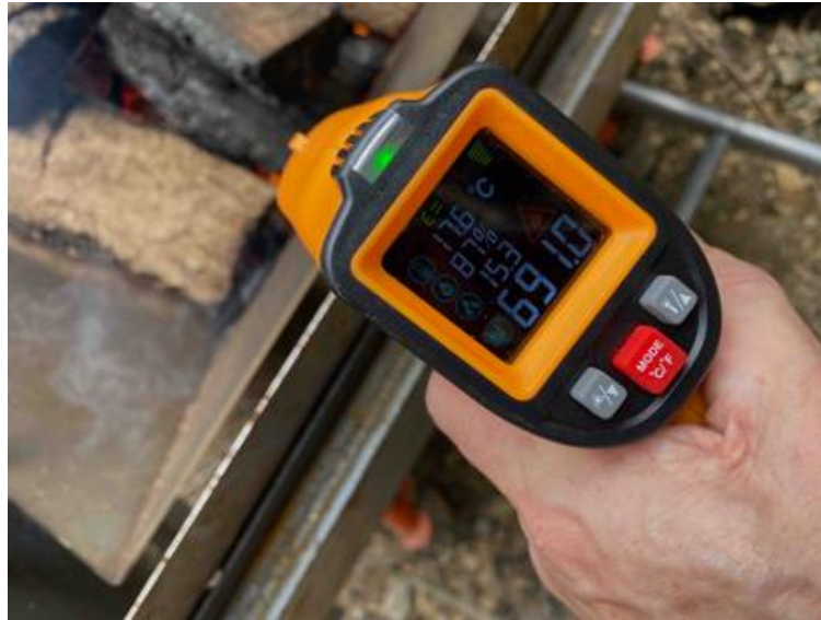
Figure 13. At this stage, the temperatures within the kiln can be routinely above 600 °C. In this particular measurement: 691 °C which is at the high end of target. With experience, temperatures within the kiln can be gauged by the colour.
