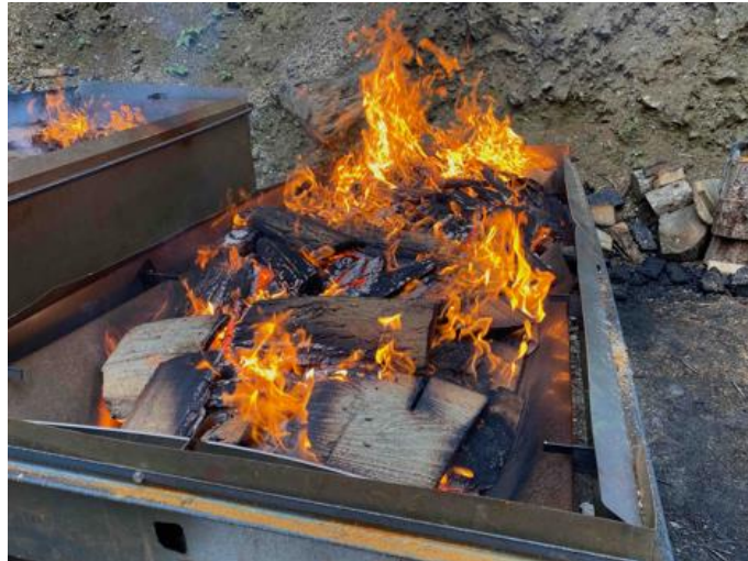
Figure 15. Kiln close to capacity, and ready to stop.
