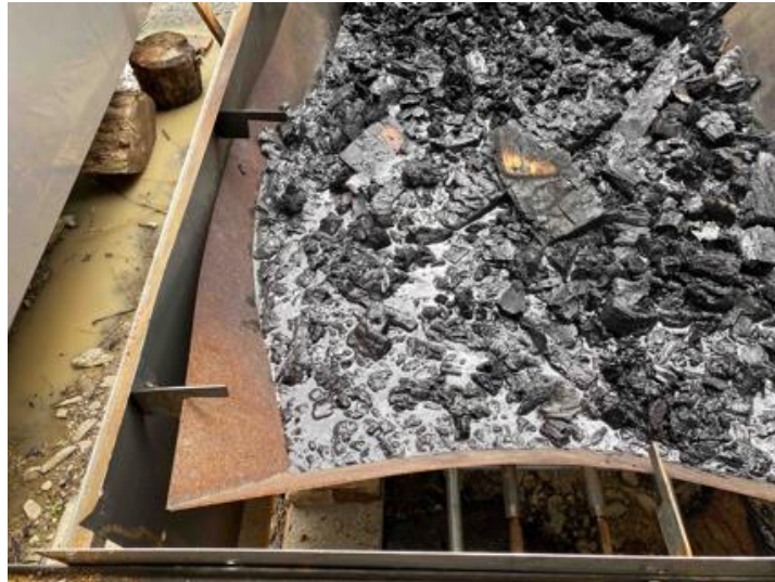
Figure 17. End of quench. All biochar has been quenched and the pyrolysis stopped. Some feedstocks at the surface will not have been pyrolyzed, because they were added near the end to keep the heat in. They may be removed at this stage. If left out to dry they can be used as feedstock in the next cycle.
