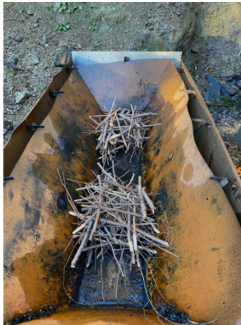
Figure 8. kindling material placed in the kiln.
