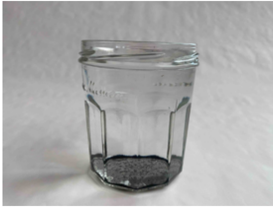
Figure 19. A typical sample of water drained from the kiln. Overnight a fine layer of microscopic biochar particles settles out, and the water remaining is extremely clear.
