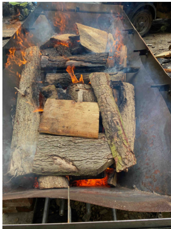
Figure 12. New layer added, trapping heat and the pyrolysis process within.
