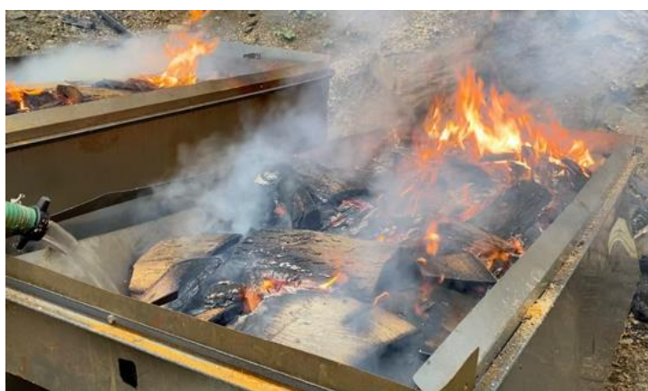
Figure 16. Pouring in quench water (gravity fed).
